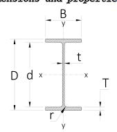
Sizes based on British Steel Section 203 x 102 x 23 UB BS EN 10365:2017 Depth of UB section:
