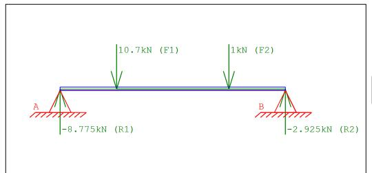
UB supported at both ends 2 equi-spaced loads applied to beam
