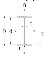
Sizes based on British Steel Section 203 x 102 x 23 UB BS EN 10365:2017 Depth of UB section:
