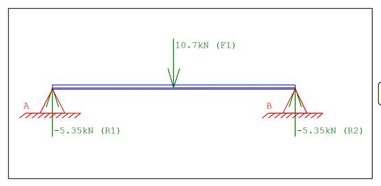
UB supported at both ends load F1 applied to beam
