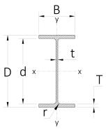
Sizes based on British Steel Section 203 x 102 x 23 UB BS EN 10365:2017
