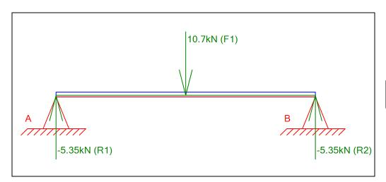
CHS supported at both ends load F1 applied to beam
