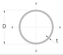
Sizes based on Steel Construction Insitute Section 219.1 x 8.0 CHS BS EN 10219-2:2006 Outside Diameter of CHS: D := 219.1 mm
