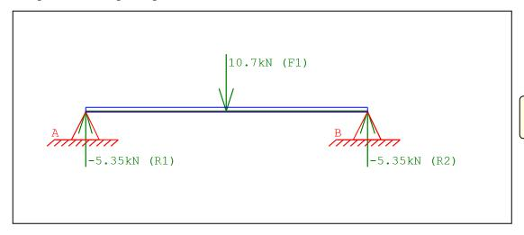
CHS supported at both ends load F1 applied to beam
